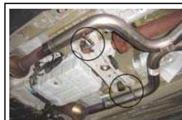
**Note:** Any 2008-10 V6 or GT owners with vehicles sent from the factory without the two transmission cross-member exhaust hangers must purchase them from your local dealer and install them in the proper mounting hole to insure your new x-pipe will fit properly.
