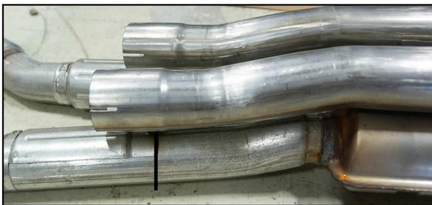
4. Once you are confident that your marks are in the right place cut the factory exhaust system along those lines. Cut as square as possible and de-burr any sharp edges after the cutting process. If your factory exhaust is equipped with heat shields, they must be removed where they interfere with the delete pipe slipping onto the stock system.
