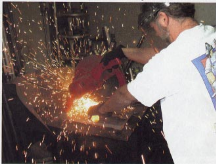
Because our '55 was sporting a few odds and ends, Lee over at The Muffler Man had to hack into a few of our Pypes to get the best fit possible.
