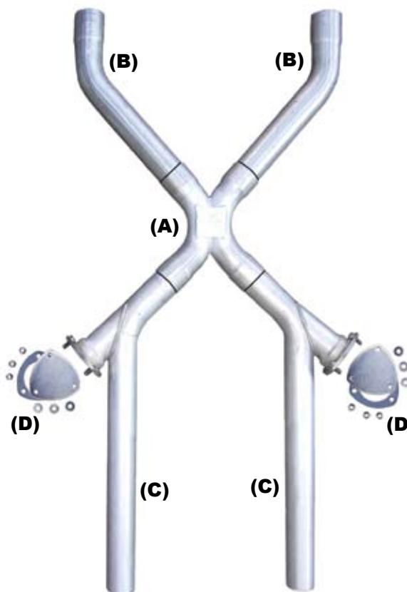
1. This five piece kit is a universal kit produced to fit many applications. Measuring and cutting will be required. The x-pipe is designed to connect after your collector reducers or down-pipes under the transmission cross-member.
